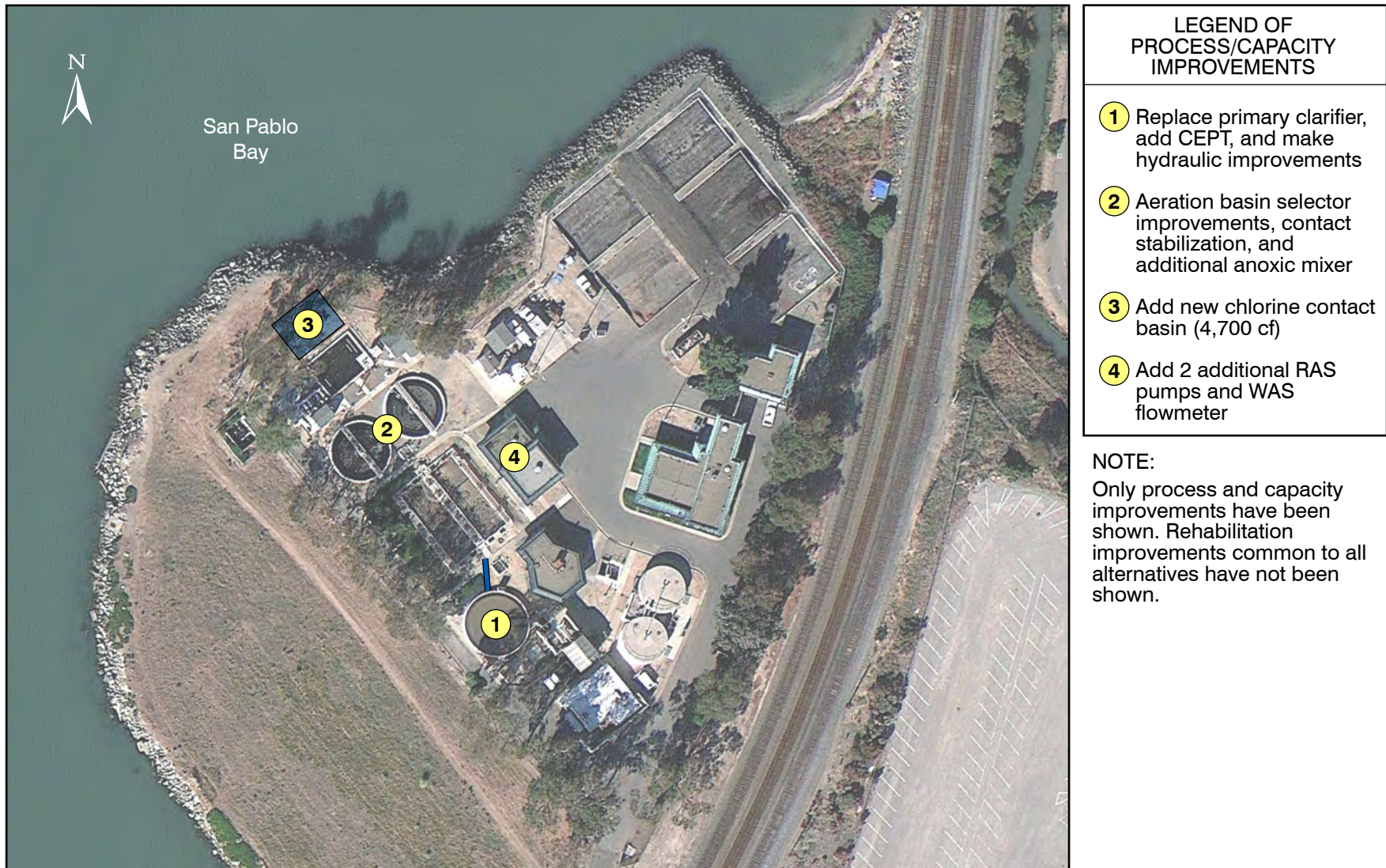
Figure 6.4 ALTERNATIVE 2 - MEDIUM I&I REDUCTION WWTP IMPROVEMENTS COMPREHENSIVE WASTEWATER MASTER PLAN RODEO SANITARY DISTRICT
